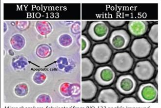
Microchambers, fabricated from BIO-133 enable improved resolution in live cell imaging.
