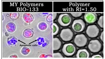
Microchambers, fabricated from BIO-133 enable improve resolution in live cell imaging.
