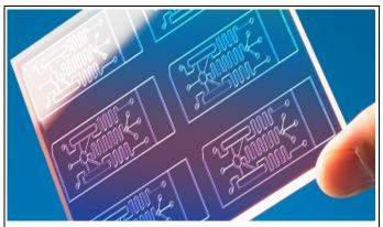
Microfluidic devices, fabricated from MY-133-V2000 reduce artifacts in fluorescence and quantitative phase imaging.
