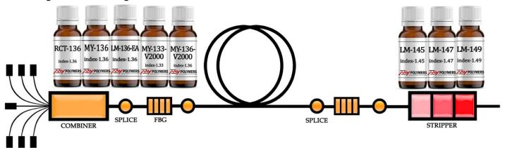
Drawing #2 shows a typical schematic diagram of an Erbium Doped Fiber Amplifier (EDFA). The splice points require recoating. Likewise, re-coating is required for most components such as couplers, combiners, and splitters.
